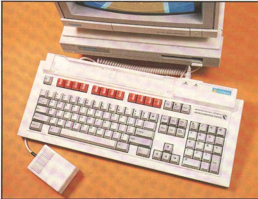
Red keys remain but the keyboard is now an international standard layout
